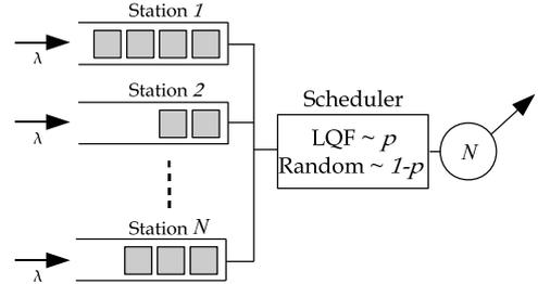
Figure 2: Centralized Scheduling with Communication Constraints
