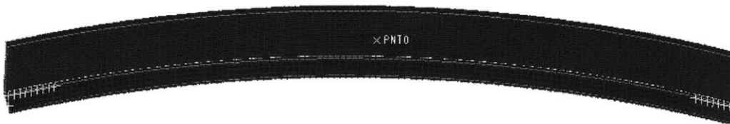
Figure 5.41 Shrinkflange R = 120" , 30 deg , Flange Width = 2"
