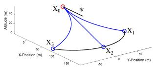
Figure 4. Diagram of the reachability set approximation for  $N_P=3$  and  $\tau=t_P=rac{\pi}{2\omega_{\max}}$ .
