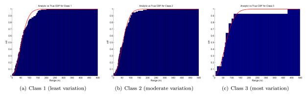
Figure 1. Comparison of miss distance CDFs for the wind profiles (blue) and tuned wind model (red) for each wind class.
