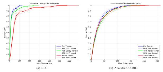
Figure 10. Miss distance CDF for BLG and Analytic CC-RRT on various terrain scalings, over 500 trials.
