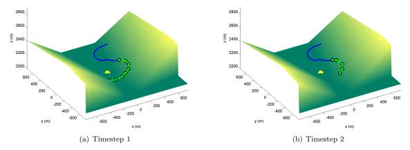
Figure 7. Trajectory planned using RRT with mean wind, during the first two timesteps. Trajectory history is shown in blue, while the current, feasible path being executed is shown in green.
