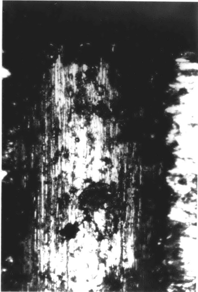
Figure 12 – Abraded and pocked contact tip surface (40x)
