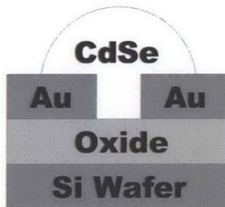
Figure 079: Schematic of a half-printed CdSe FET. The top Au source/drain electrodes were fabricated by liquid embossing.
