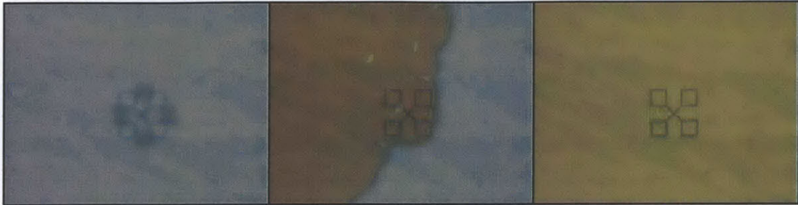
Figure 063: Three optical images showing the alignment mark of the stamp coming into contact with the liquid and the previously patterned metal film. (Time proceeds from left to right.)
