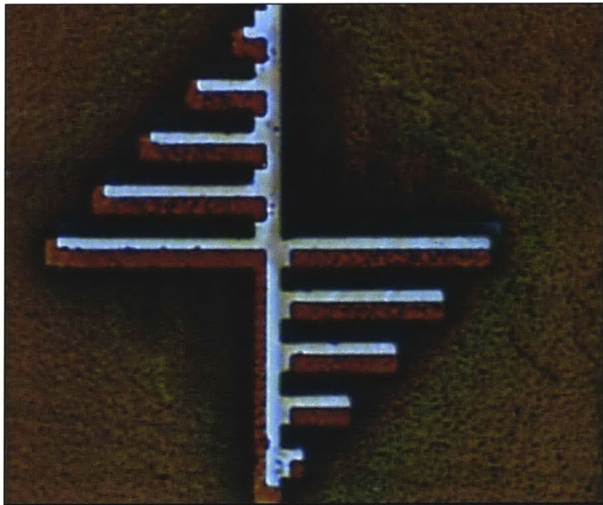
Figure 062: Optical image of 4 layers of alignment marks aligned to within 2 \mu m.
