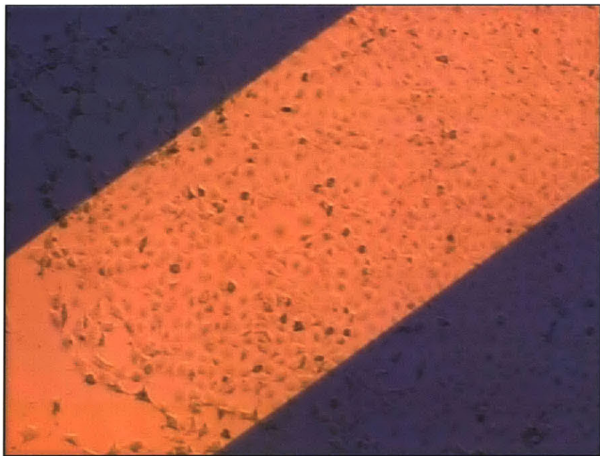
Figure 118: Cell growth on Au and SiO 2 . This was the control wafer and thus was not coated with a SAM.
