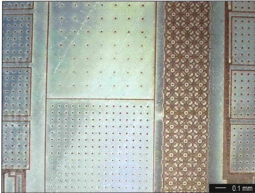
Figure 018: Optical image of 3µm patterns fabricated in Ag.
