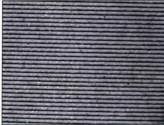
Figure 009: Optical image of metallic grating with 3\mu\text{m} periodicity fabricated in Au.
