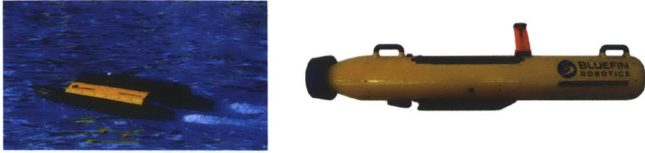
Figure 3-2: Left: A Kingfisher M200 Unmanned Surface Vehicle (USV) and Right: a Bluefin-9 Unmanned Underwater Vehicle (UUV).
