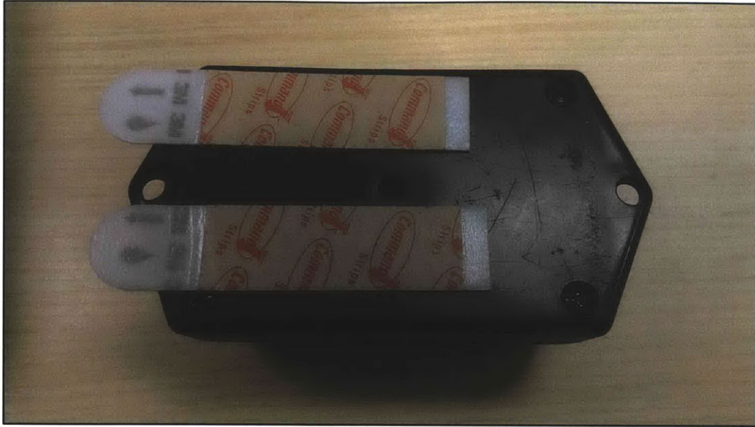
Figure 52: CAPTCHA Attaches to Equipment Via Command Strips.
