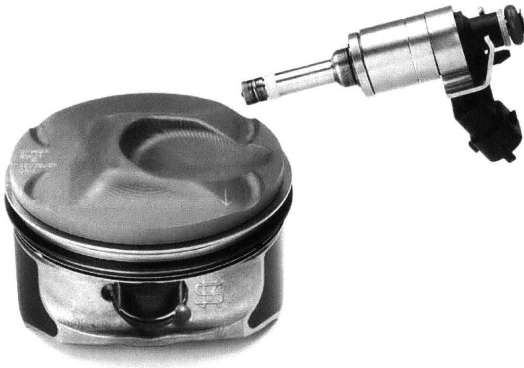
Figure 2-5: A common piston shape for cold-start features a bowl oriented to the fuel injector such that the piston geometry redirects fuel, alters fuel-air mixing and induces favourable center-rich, perimeter-lean fuel stratification. Establishing a rich mixture towards the spark plug improves the early stages of ignition and flame growth, which in turn, reduces the cycle-to-cycle variability of operation at late ignition timing. Image credit:[2]
