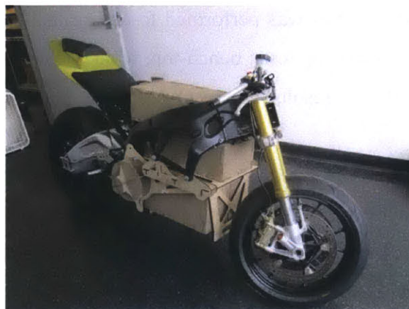
Figure 3.7: The frame and battery assemblies were prototyped using cardboard and wood cut on a laser-cutter according to the CAD files.
