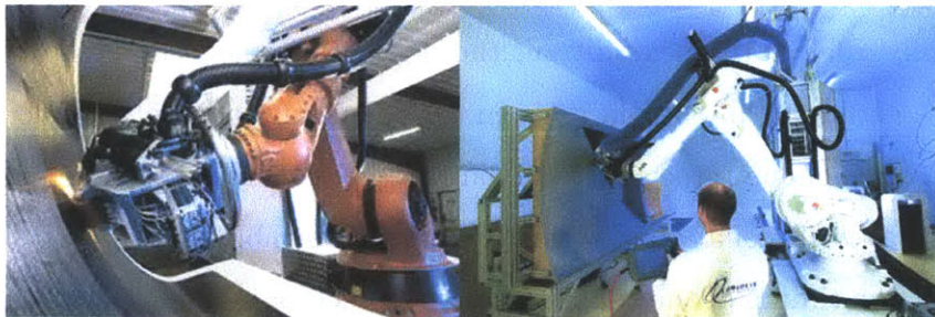
Figure 1-5: 'Right-sized' robot systems being developed for drilling large aircraft structures
