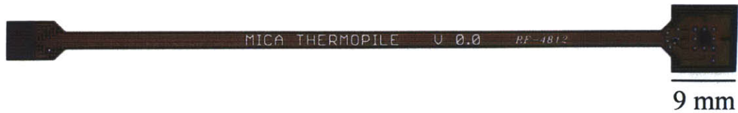
Figure 1-7: MICA external thermopile for IR temperature measurement.
