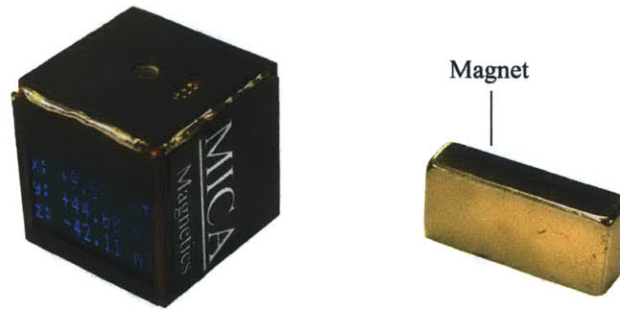
Figure 1-4: MICA 3-axis magnetic field sensor, measuring the field of a magnet.
