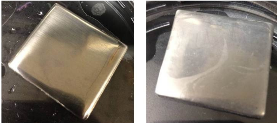
Figure 6.8: Images of polished (left) and etched (right) Ti6Al4V coupons.
