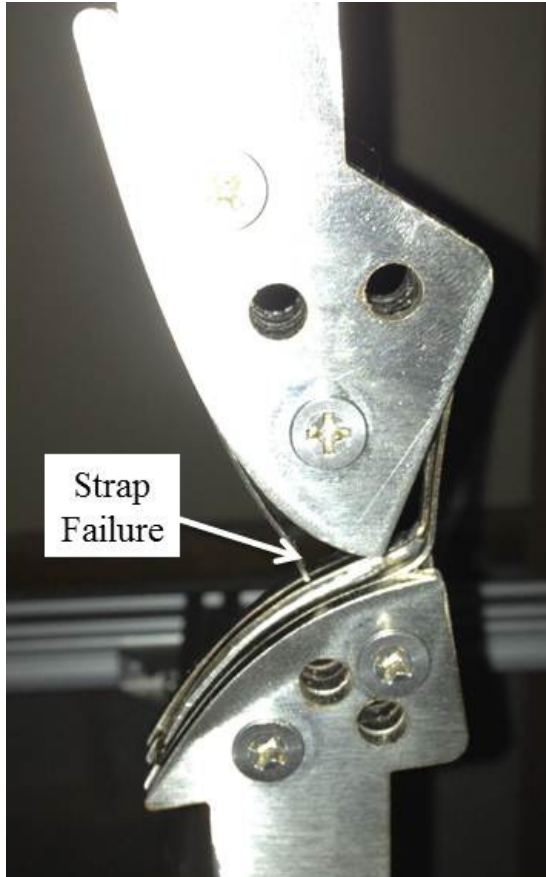
Figure 5.16: Image of failure in the middle strap.
