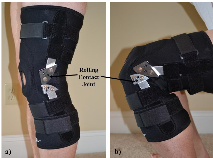
Figure 5.15: Rolling contact knee brace joint in extended (a) and flexed (b) positions.
