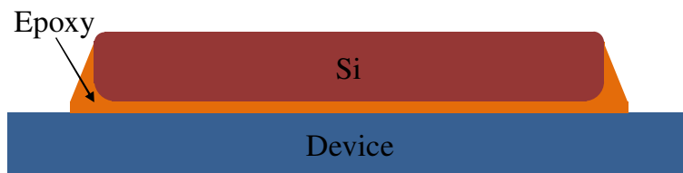
Figure 5.30: Schematic of delamination step, showing the piezoresistor cured to the device surface after the stamp is removed and the adhesive wax is cleaned off from the surface.
