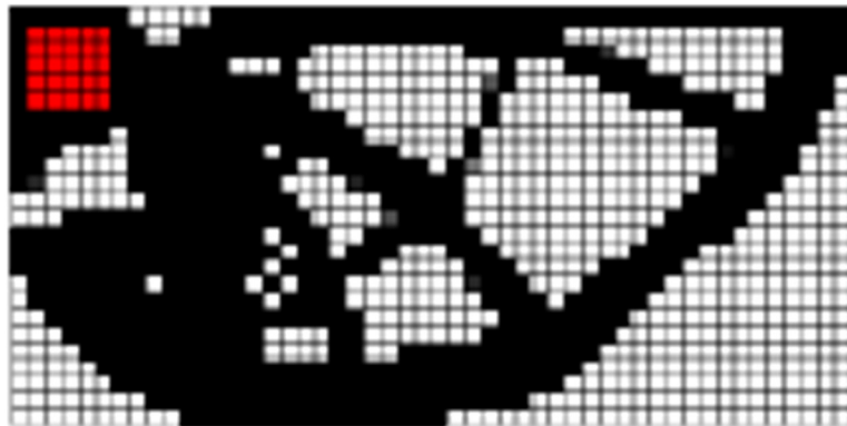
Figure 1.13: Iterative topological optimization of a force sensing cantilever (black) with piezoresistive sensor (red). The force is applied at the top right of the cantilever [38].
