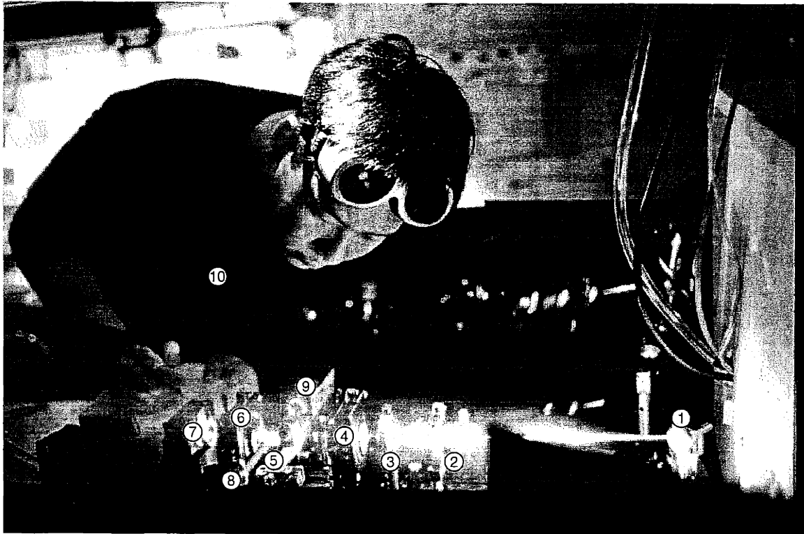
Figure 3-17: A photograph of M3, the third microscope prototype. Indicated are (1) a fold mirror bringing laser power from the argon laser (not shown); (2) a spatial filter assembly; (3) the diffractive beam splitter in a rotating mount; (4) a field lens on a five-axis gimbal mount; (5) a non-polarizing beam splitting cube; (6) microscope objective lens; (7) MEMS mirror array; (8) fold mirror to fiber grid array chuck (not shown); (9) a beam stop for the unwanted reflection from the beam splitting cube; and (10) Stan Hong.
