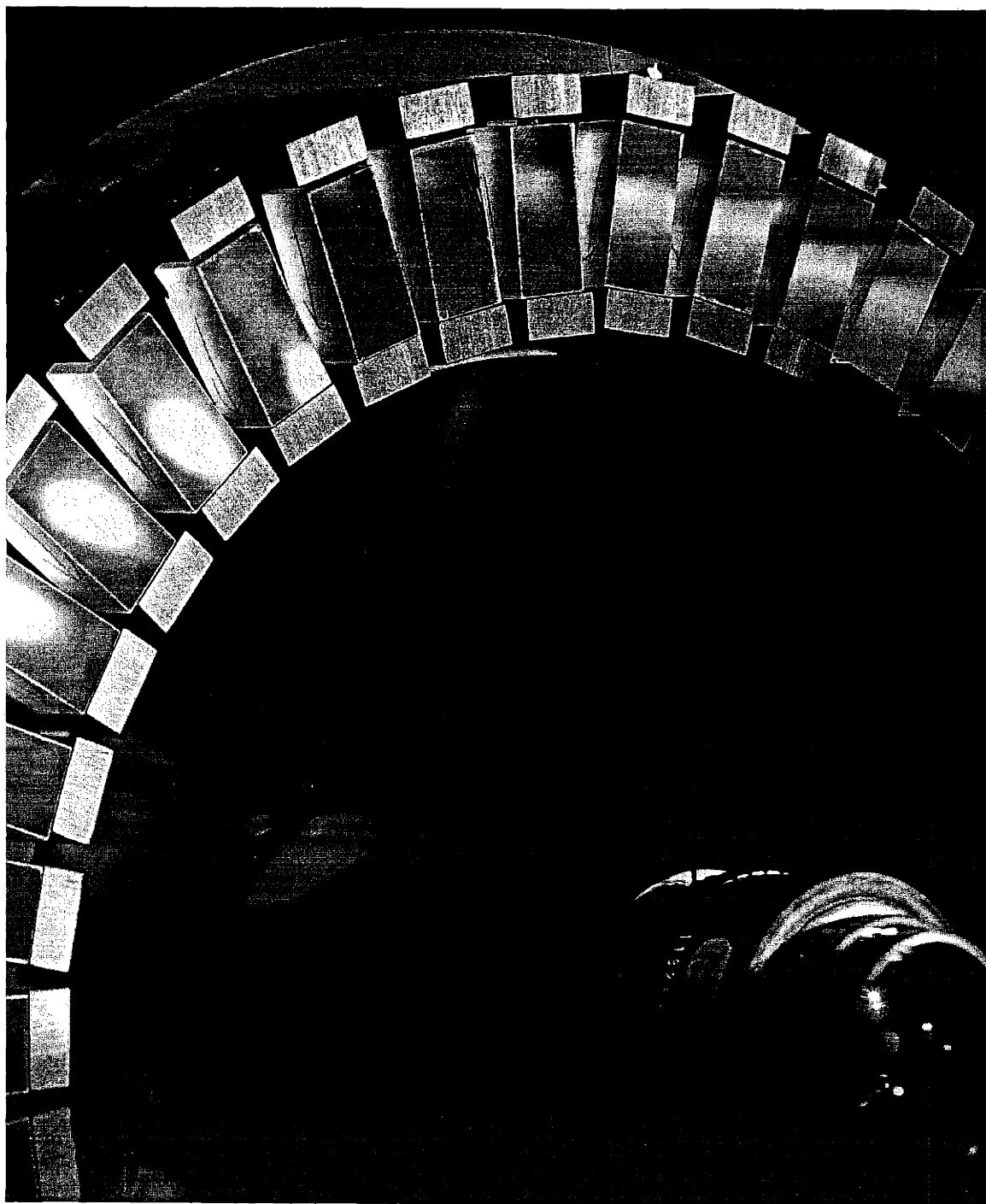
Figure 1-2: In one of the microscope prototypes for this thesis, a standard camera lens (lower right) was augmented by a ring of diffraction gratings—using Synthetic Aperture Microscopy ideas to boost its resolution performance a thousand fold. The working distance, field of view, and depth of field were not reduced by the upgrade. Shown approximately life-size, the combination of lens and large ring (which is mostly cut off) provides the performance of a mathematically perfect lens as big as the large ring.
