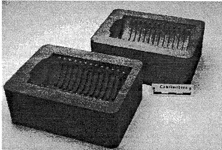
Figure 1.6: Green (foreground) and post-processed injection molding tool made with the 3D Printing process.
