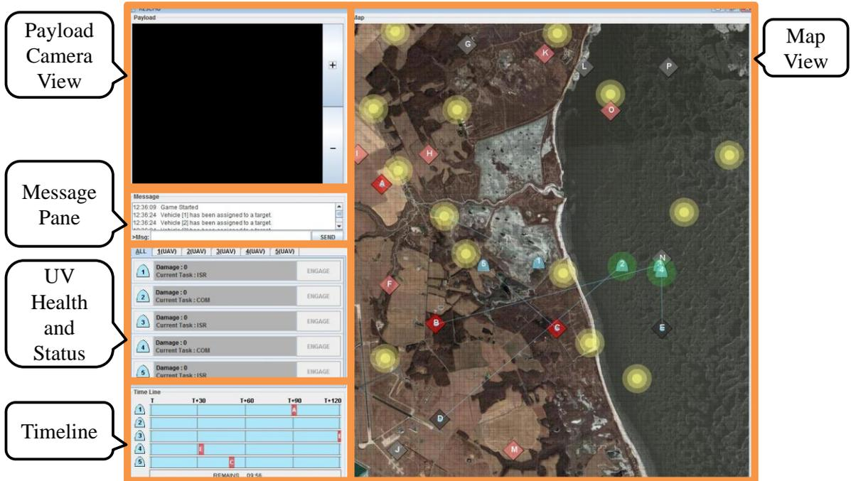
**Figure 4. Annotated screenshot of the operator display – Research Environment for Supervisory Control of Heterogeneous Unmanned Vehicles (RESCHU)<sup>15</sup>**
