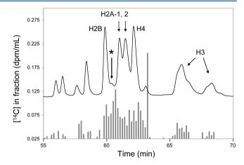
**Figure 2.** HPLC analysis of histones isolated from [<sup>14</sup>C]3,5-DMAP-treated cells showing UV detector response (continuous trace) and <sup>14</sup>C concentration in collected fractions.
