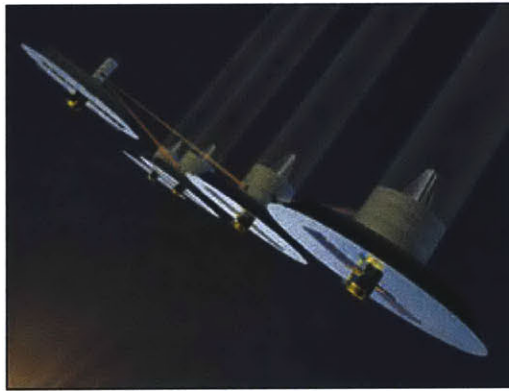
Figure 2.3 Artists rendition of four TPF spacecraft flying in formation, observing a distant solar system (white = starlight, red = metrology). [Beichman, 1997-1998]
