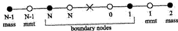
Figure 4-3: Schematic representation of the numerical grid near an interface. The interface is indicated by a cross, the nodes by solid dots and the cell centers by open dots. We note that, in fact, the rightmost node (i.e.: N ) of the left domain, the leftmost node (i.e.: 1) of the right domain, and the interface are the same point in space, but (because they play different roles in the numerical algorithm) they are represented separately in the picture. Similarly, there is no cell N belonging to the left domain, nor is there a cell 0 belonging to the right domain, but (for reasons, explained in the text) these ghost cells are introduced by the numerical algorithm — they represent extensions of the material phases on each side of the interface, to the other side. In space, the N -th (ghost) cell of the left domain is actually to the right of the interface, and the 0-th (ghost) cell of the right domain is actually to the left of the interface.
