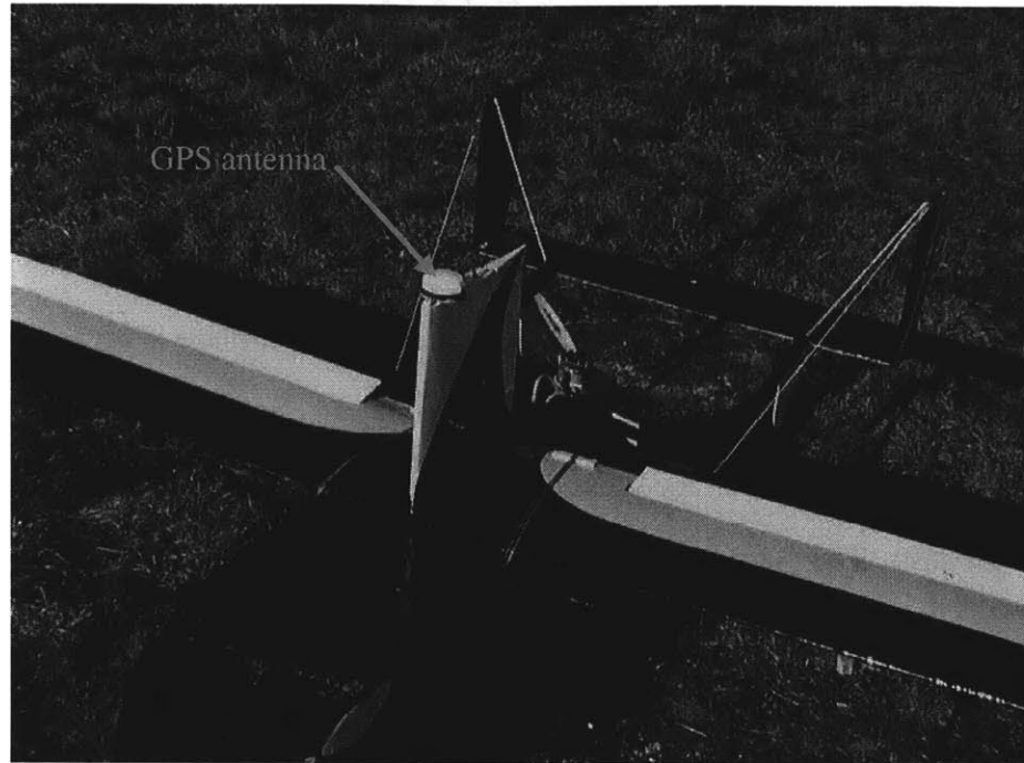
Figure 3.17 Position of the GPS Antenna on top of the Mini Vehicle
