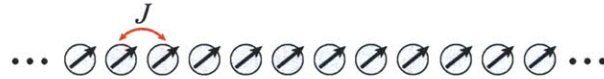
Figure 4-3: Dipoles of many molecules in semi-head-to-tail geometry. Each molecule is treated as a point dipole with nearest-neighbor interaction strength J .
