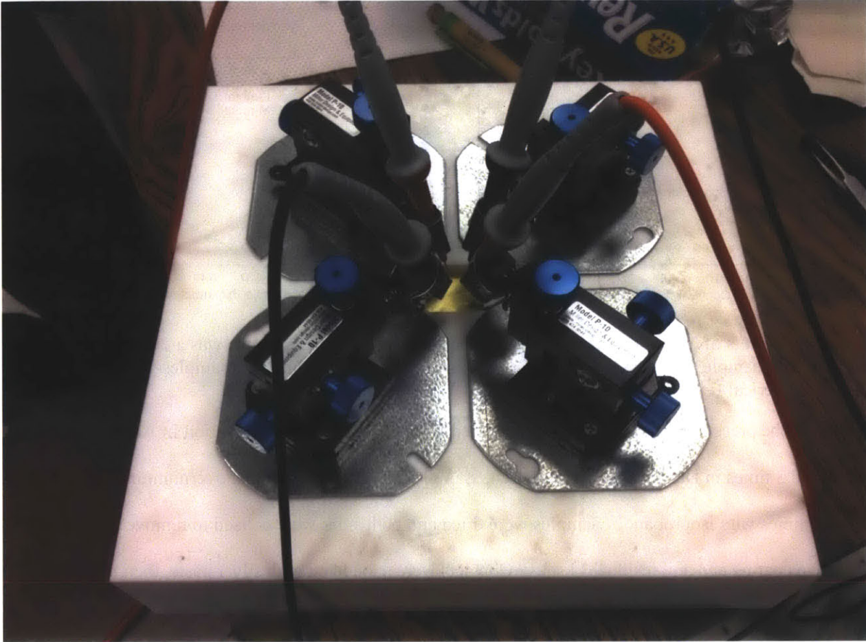
Figure 5.4: Custom-built four-point probe setup used to measure sample conductivities.
