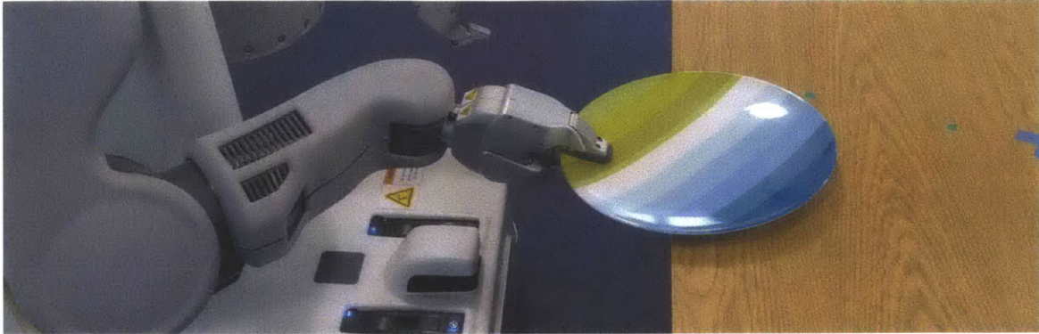
Figure 4.1: We assume the plate can only be grasped at a single position on the table.
