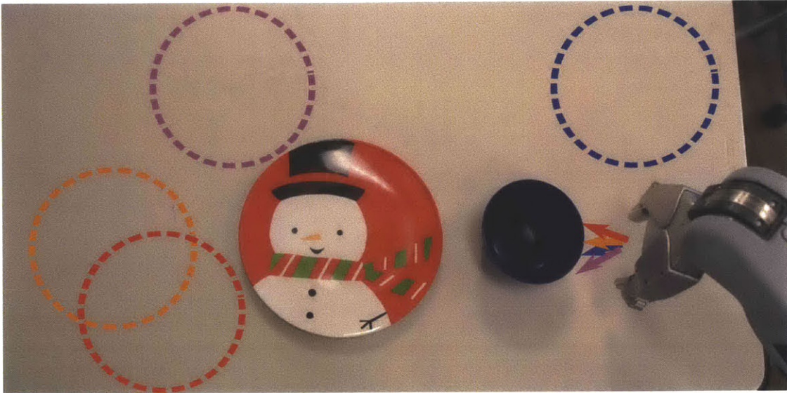
Figure 3.4: An illustration of the failure of the non-holonomic RRT in the Plate Pushing World. The bowl is a fixed obstacle and the initial configuration is shown in the photograph. Every straight line path from the robot’s initial configuration to any configuration in which the robot’s gripper is in two-point contact with the plate is blocked by the bowl. A number of samples for the plate (the sample for the robot is irrelevant and not shown to avoid clutter) are shown in different colors. The corresponding pieces of path added to the tree are shown as solid lines in the corresponding colors. Because we have zero probability of sampling a configuration in which the plate is in its initial configuration, the first part of the trajectory returned by the empty space planner is always a straight line to a configuration in which the robot’s gripper is in two-point contact with the plate. Therefore, with probability one, the algorithm never adds a configuration to the tree in which the robot is pushing the plate.
