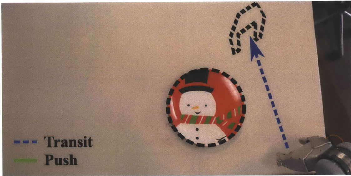
(a) If the plate's configuration in the final configuration matches the plate's configuration in the initial configuration, the empty space planner returns a single transit from the robot's initial configuration to the robot's final configuration.
