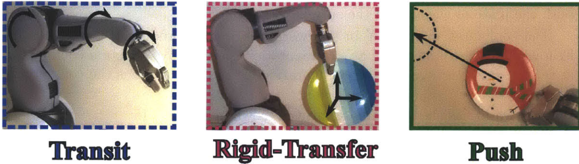
(a) The primitives available in the Push World. The robot can move by itself ( transit ). It can move the rigidly grasped plate ( rigid-transfer ). It can push the plate along the ray connecting the center of the gripper to the center of the plate when the gripper is in two-point contact with the plate, the plate rests on a supporting surface, and the gripper can move along this ray without moving the robot's base ( push ).
