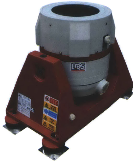
Figure 5-1: Typical shaker table for energy harvesting applications. The one shown in the figure is the LDS V406 made by Bruel and Kjaer.
