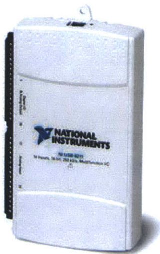
Figure 5-6: NI USB-6211 multi-function DAQ made by National Instruments. The box provides automated signal generation and data acquisition for the harvester system experiments.
