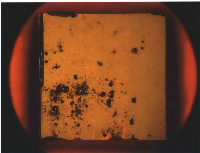
Used and Damaged SBR
