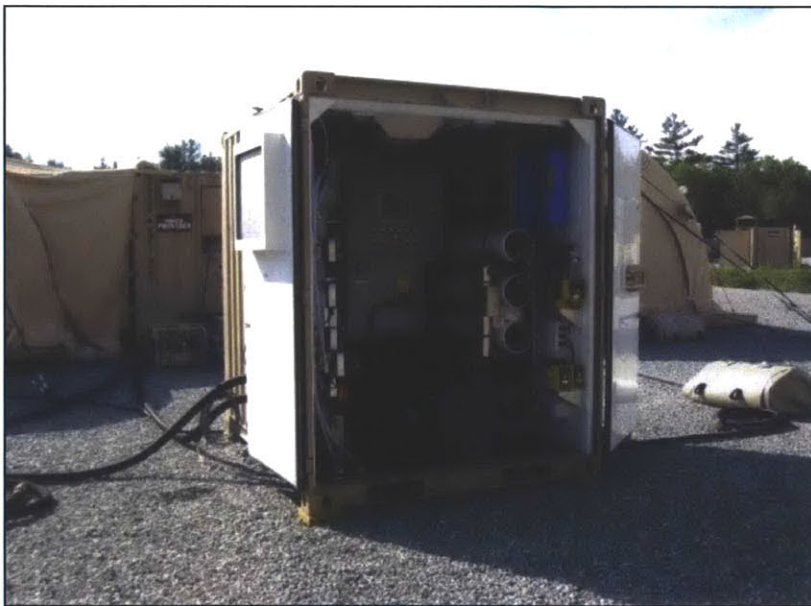
Figure 12. Shower Water Reuse System [23]
