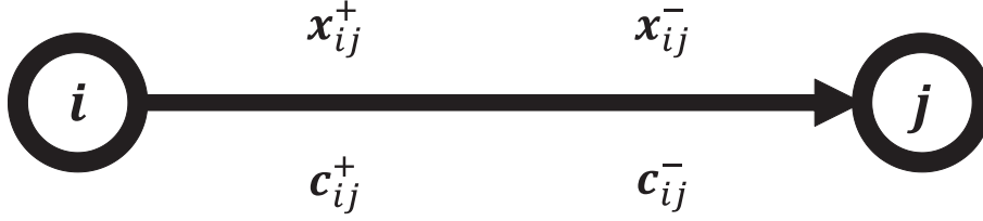
Figure 2-2: Outflow \mathbf{x}_{ij}^+ , inflow \mathbf{x}_{ij}^- , and unit costs for outflow \mathbf{c}_{ij}^+ and inflow \mathbf{c}_{ij}^-
