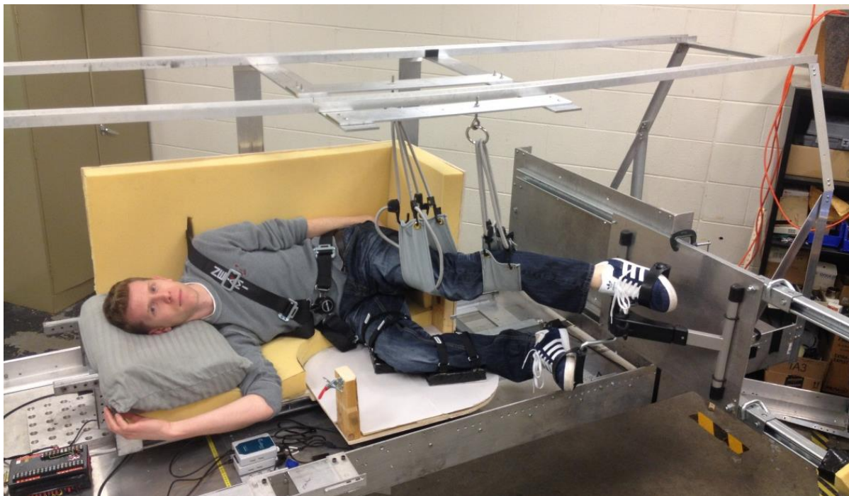
Figure 18- Leg cuff concept mockup on centrifuge (front vertical leg cuff support beam not shown)
