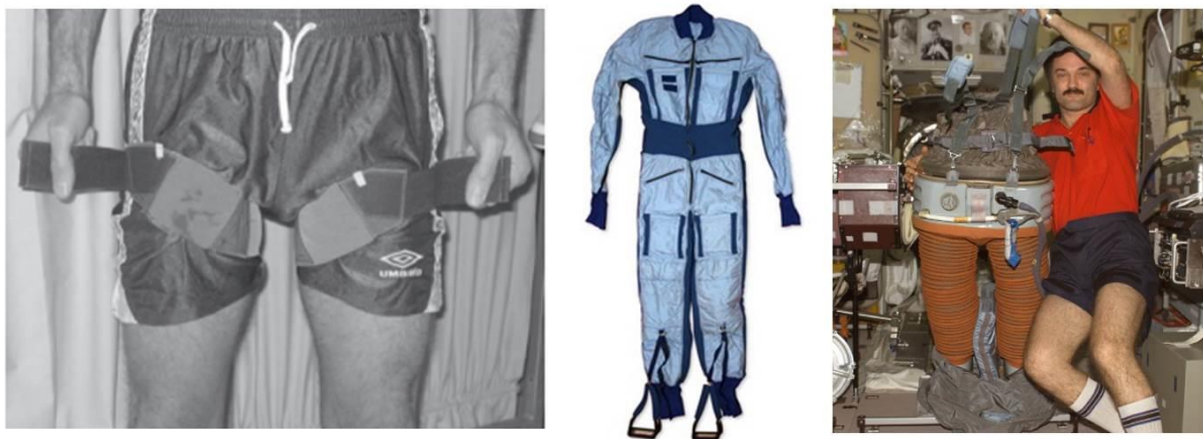
Figure 3- ISS countermeasure devices (left to right): thigh cuffs, Penguin suit, and LBNP suit [10,32], (NASA)
