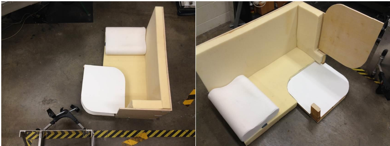
Figure 15- Seat and ergometer ground mockup in operational configuration (left) and with upper leg plate raised for subject seating (right)
