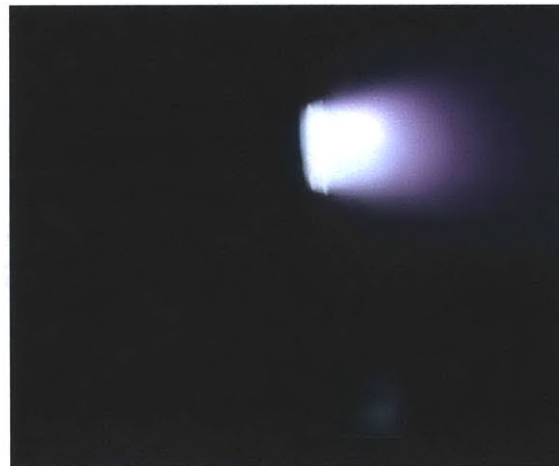
Figure 3-7: The CCFT firing with 4 sccm Xe flow and 300 V at the anode.
