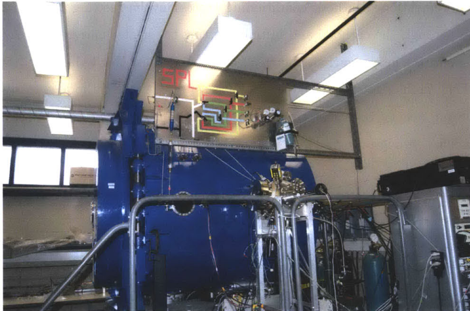
Figure 3-2: The Space Propulsion Laboratory Astrovac vacuum chamber. The chamber, used for the CCFT testing, is pumped by two cryopumps and one mechanical roughing pump.
