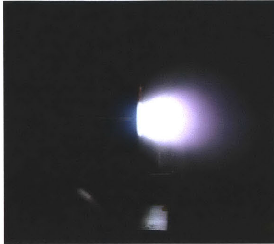
Figure 3-6: The CCFT firing with 4 sccm Xe flow and 200 V at the anode.
