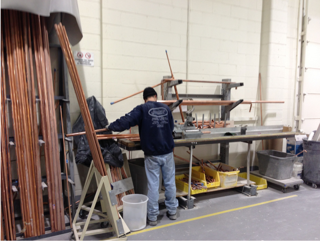
Figure 3.3-6: Waste reduction through accurate cutting of pipes (Eggrock Modular Solutions, 2013)
