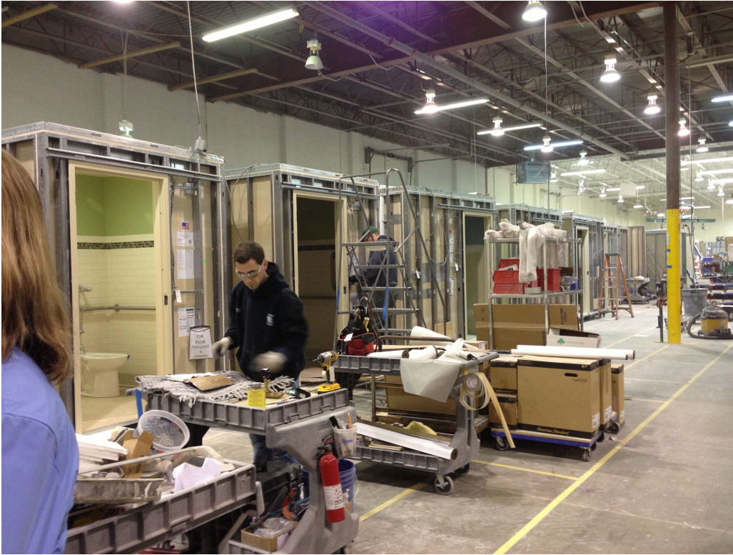
Figure 3.3-7: Increased efficiency by concentrated equipment around the workers (Eggrock Modular Solutions, 2013)
