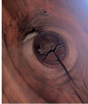
**Figure 3.7: Local cracks surrounding a knot in a wood specimen**
