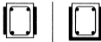
**Figure 3.18: Reinforced concrete specimens using FRP bonded externally to the side of the specimen or in a U shape referred to as U jacketing (Chen and Teng, 2003).**
