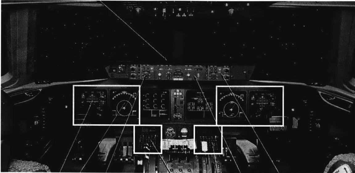
Fig. 5: View of the MD-11 cockpit. The display units where VG sends feedback information are highlighted (white squares).
