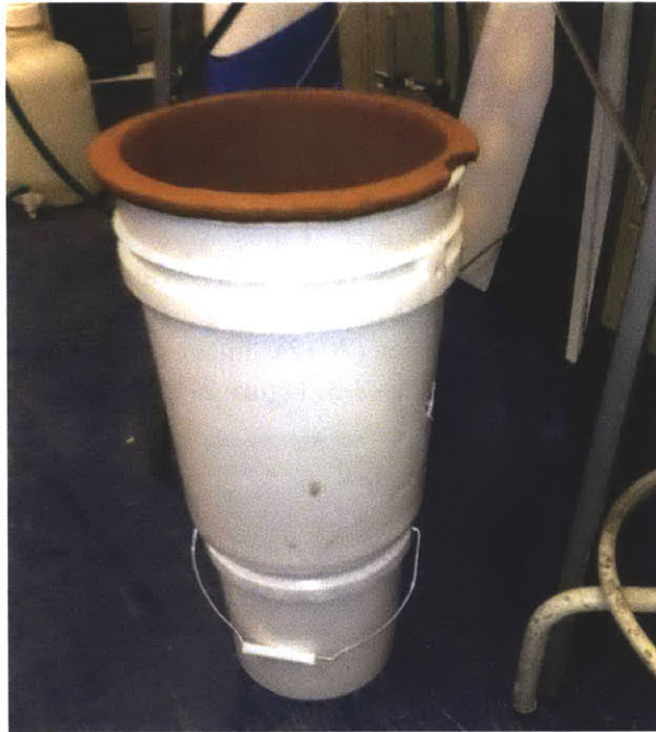
Figure 2-2: Lab testing of flowerpot filter
