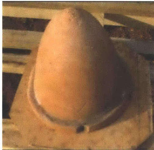
Figure 2-4: Paraboloid filter (image from Miller, 2010)
