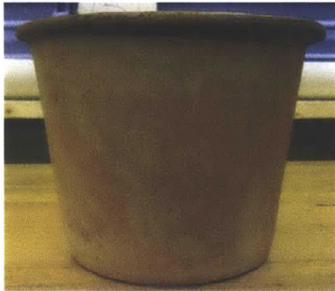
Figure 2-3: Flowerpot filter (image from Watters, 2010)
