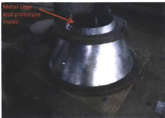
Figure 40: Metal cone around the cage, and secured with wires Figure 41: Pouring concrete
