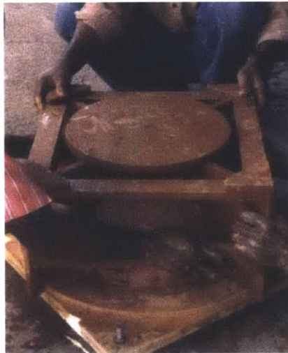
Figure 37: Rotating Item B to make the shape of the prototype filter element
