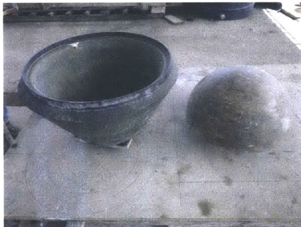
Figure 49: Finished female mold (left) and male mold (right)
