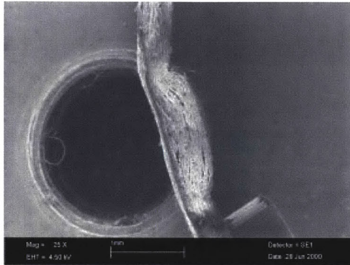
Figure 4-20: SEM image of TRIPLEX TM MD folding process (step 3) [18].
