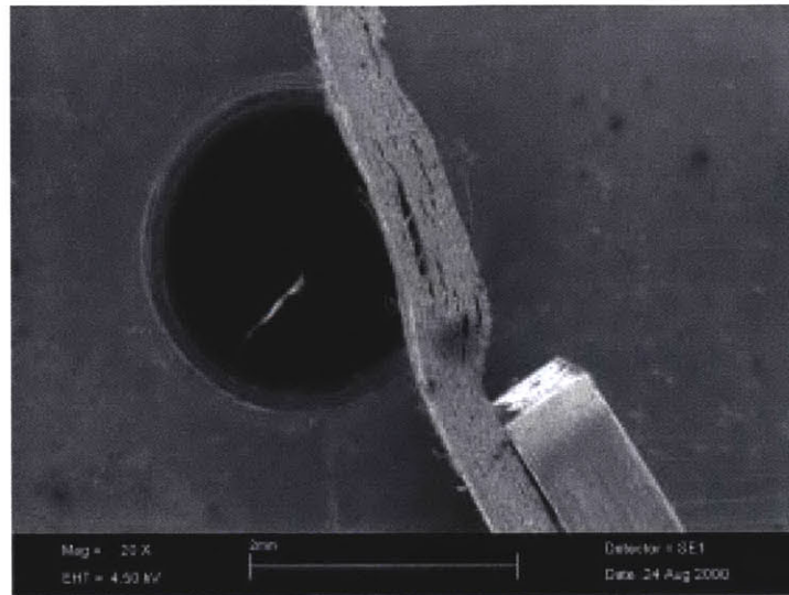
Figure 4-36: SEM image of TRIPLEX TM MD punching process at step 2 of folding (male die width 0.84mm and female die width 2.03mm) [18].
