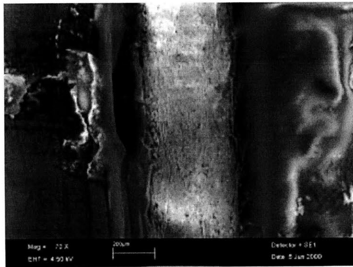
Figure 3-7: Triplex MD through-thickness SEM tension image correlated with stress-strain data obtained by Dunn [18] (Step 3).
