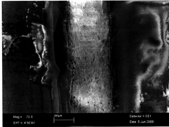
Figure 3-6: Triplex MD through-thickness SEM tension image correlated with stress-strain data obtained by Dunn [18] (Step 2).
