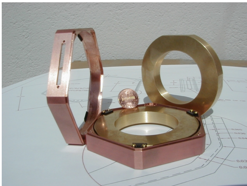
Figure 7-4: CDMSII detector holders, with placeholders occupying the detector space. The DIB cutout is visible on the empty placeholder standing on its side. Courtesy: Dennis Seitz.
