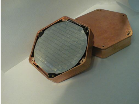
(a) Figure 3-1: Picture of a CDMSII ZIP detector. The phonon sensor side is shown in the image.
