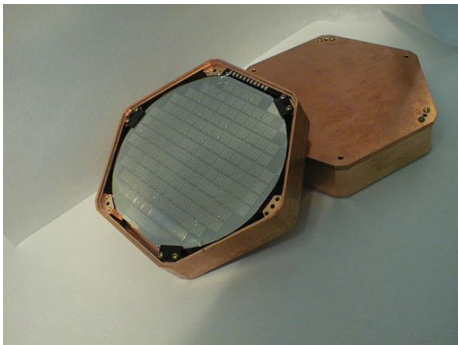
(a) Picture of a CDMSII ZIP detector. The phonon sensor side is shown in the image.
