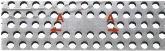
(a) Optimization on the position of one hole in L_3 cavity [5]. Q=50000 and V = 0.7(\lambda/n)^3 .
