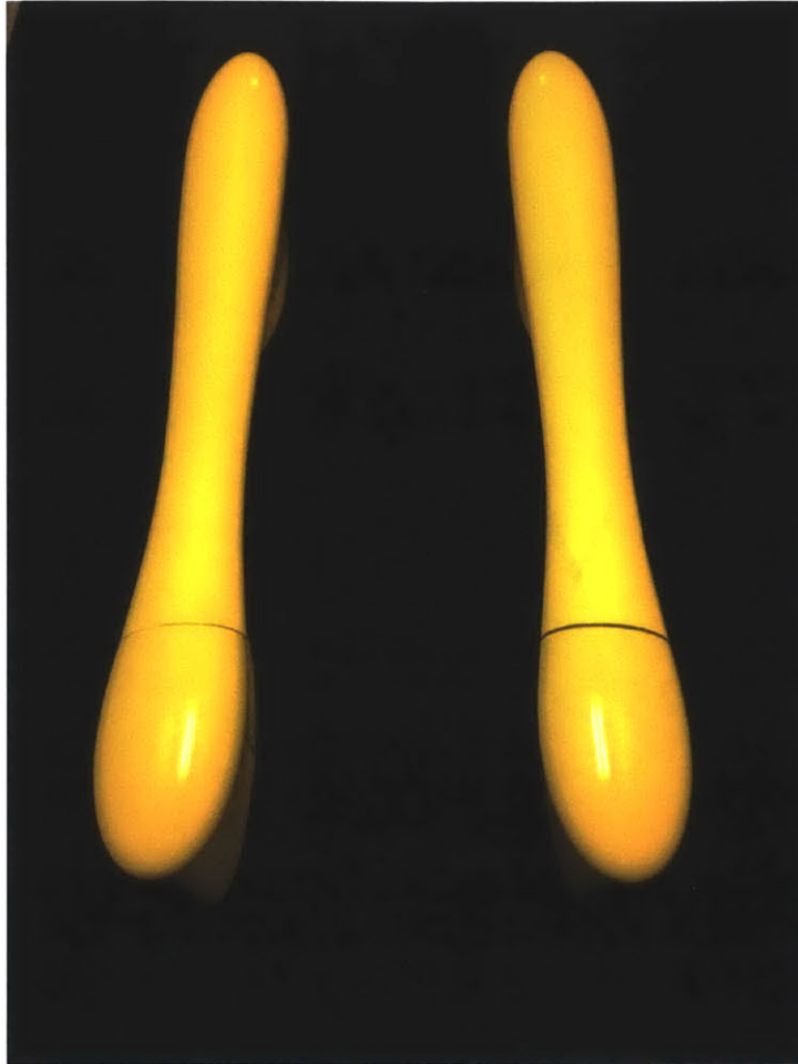
Figure 11: The completed submerged bodies. Note that the bow sections are not yet permanently attached.
