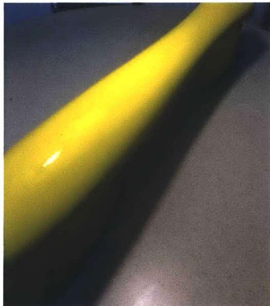
Figure 10: A close up view of the finish on the submerged bodies after several coats of polyurethane paint
