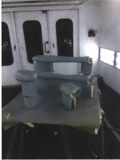
Figure 9: the submerged body pieces after being given a coat of primer in the automobile spraypaint booth
