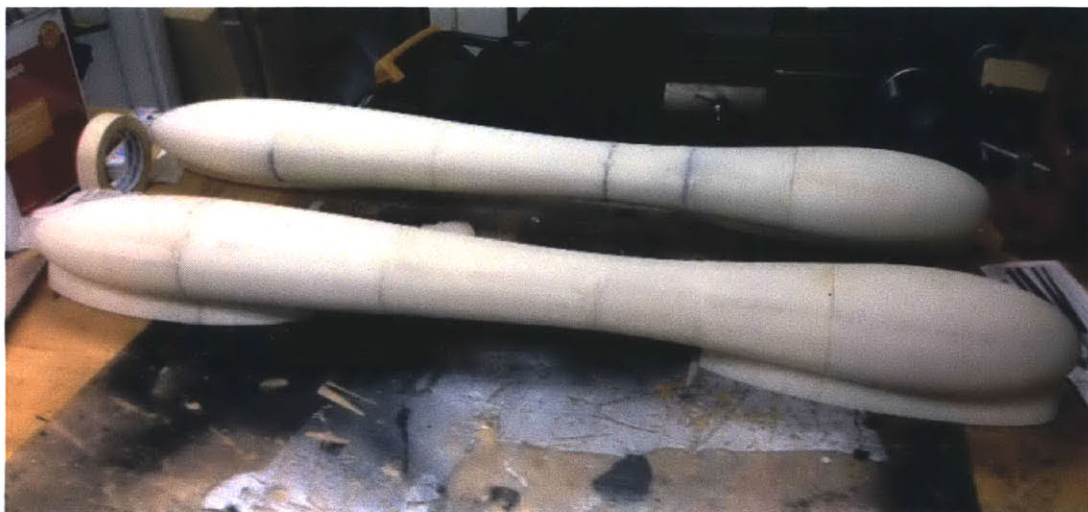
Figure 8: The assembled submerged bodies. Note the gray lines where modeling putty was used to fill in gaps.
