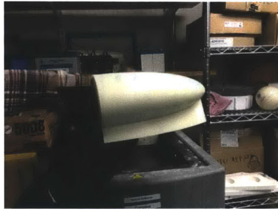
Figure 7: The stern section of the submerged bodies being removed from the acid bath
