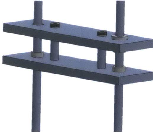
Figure 7: Dropping carriage in the vertical test apparatus.
