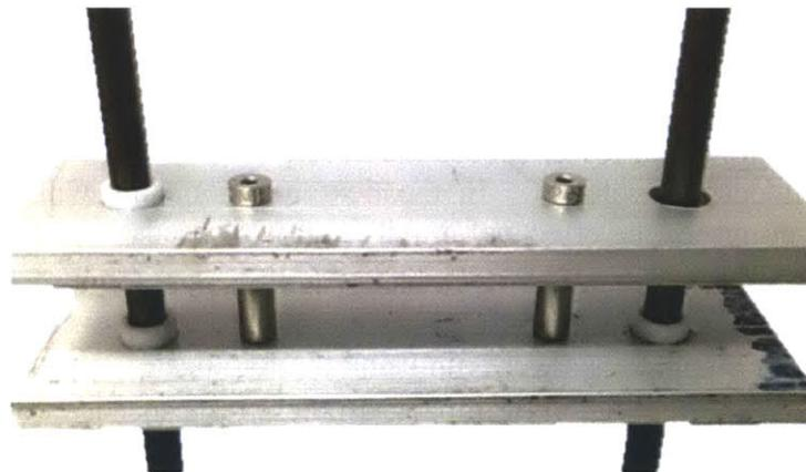
Figure 10: Dropping carriage without needle sample. Shoulder bolts, PTFE bushings, and sliding rods are shown.
