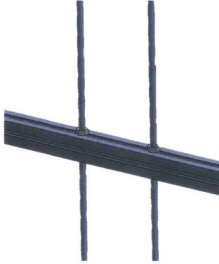
Figure 8: Top guide rail attachment to support structure.
