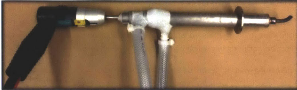
Figure 2-4. Lancom standard probe encased in concentric tube heat exchanger
