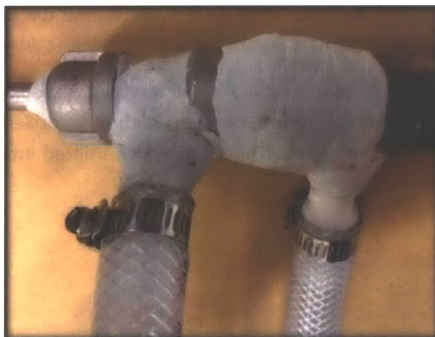
Figure 2-9. Epoxy putty supports the acetal barbed fittings at the inlet and outlet of the probe heat exchanger and seals the pipe caps from the high pressure water supply.
