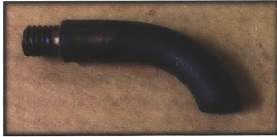
Figure 2-10. The stainless steel 10-32 threaded elbow was screwed onto the end of the probe to increase sample line flow velocity. In this image it has been blackened due to oxidation by the flue gases.
