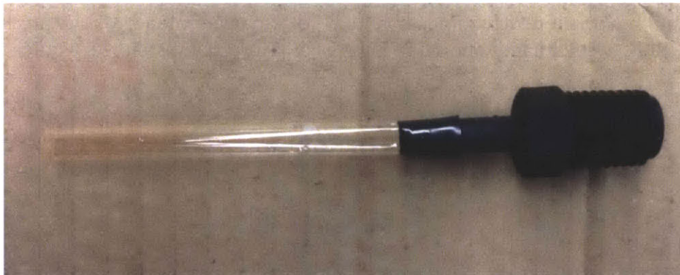
Figure 8b: Microspec tubing used as a valve prototype. Medium length piece shown, with length = 2.5 inches, outer diameter = 0.253 inches, and thickness = 0.005 inches
