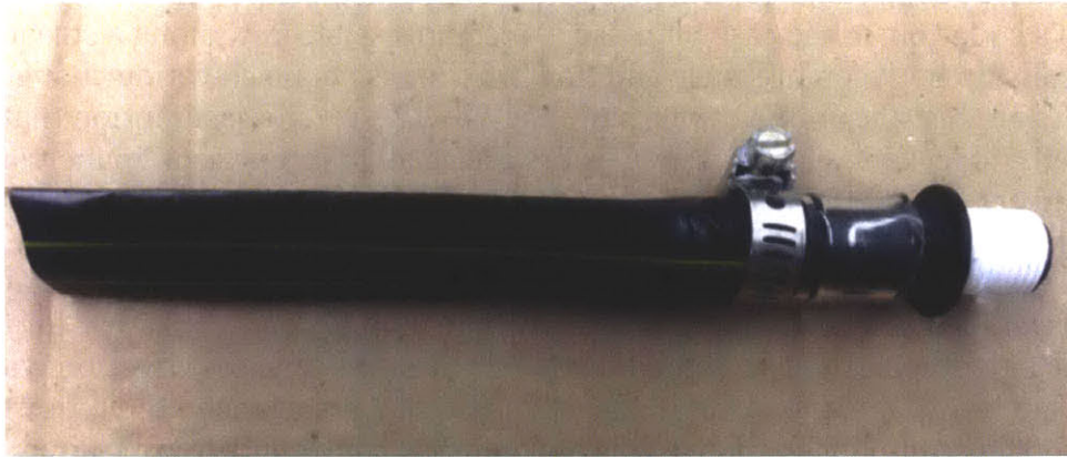
Figure 8a: Valve prototype made from tubing supplied by Jain Inc. Length = 5 inches, outer diameter = 0.65 inches, and thickness = 0.0075 inches
