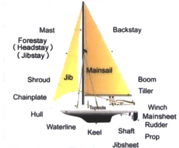
Figure 1: Diagram of the structure of a simple sailboat. 1
