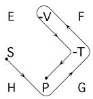
For a simple hydrostatic system
