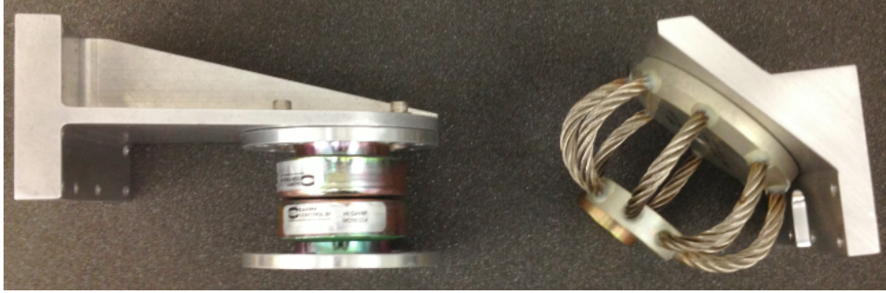
Figure 4-19: Two low-frequency damper options are being considered to isolate LMO from the rocket skin vibrations. The Barry rubber dampers (left) have a higher natural frequency than the WRI's (right).
