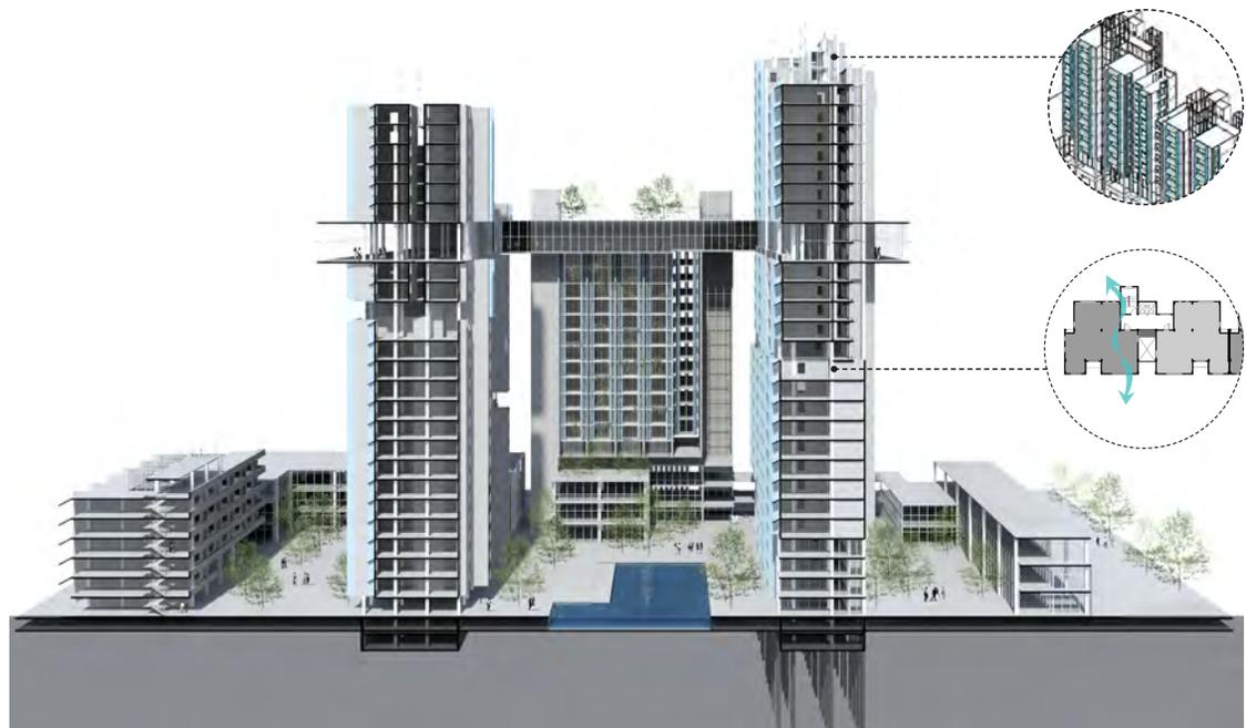
*4-0.4b Above is a tower-in-park retrofit section showing the integrated sustainability and energy strategies to enhance the livability of the tower structures, including partial erosion of the facade, stack effect with vertical natural ventilation, cooling pools in the courtyards, geo-thermal wells, and in-unit cross ventilation.*
