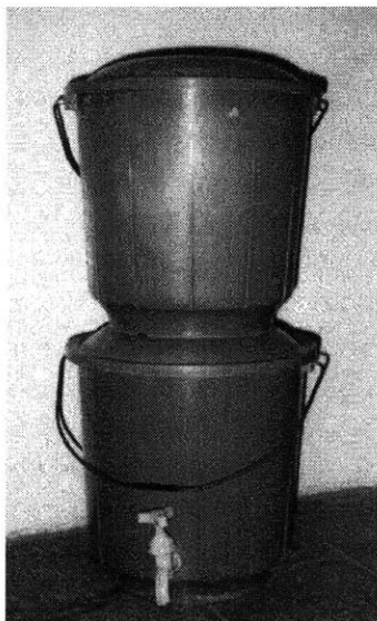
Figure 4.4: Modified-Bucket Chlorination System, with Candle Filter
