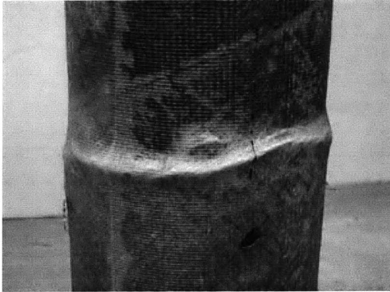
Figure 4.37 Local fiber buckling / fabric wrinkling in C1 – WA1 – SP3
