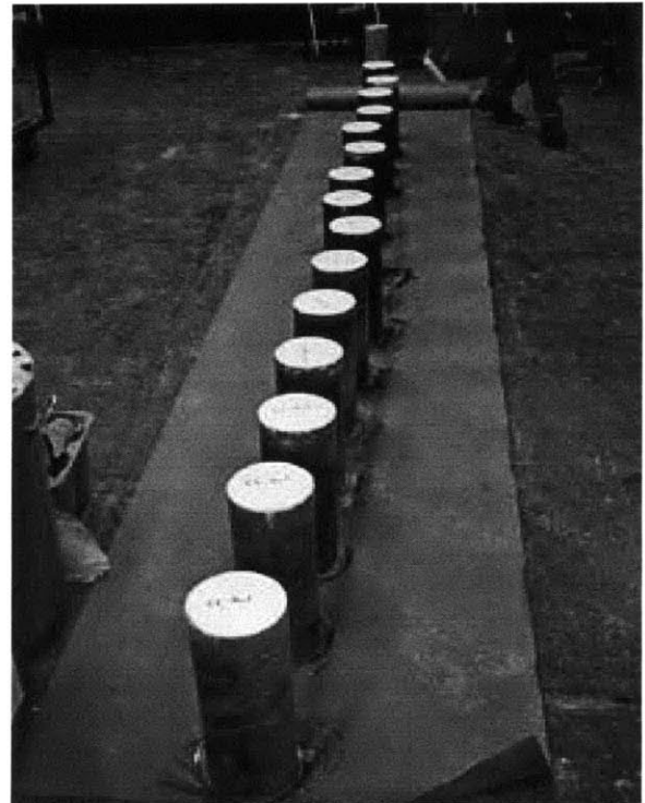
Figure 4.6 Primed cylinders under curing for at least one hour (surfaces were darkened by the prime coat)
