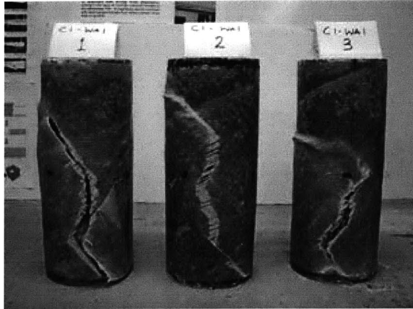
Figure 4.24 Failure mode III (C1 – WA1)
