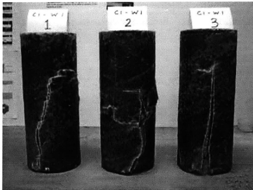
Figure 4.23 Failure mode II (C1 – W1)
