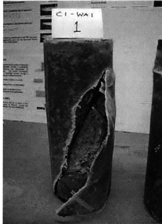
Figure 4.39 Concrete shearing fracture within fabric
