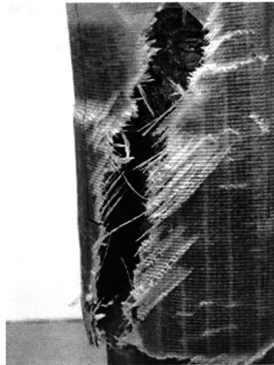
Figure 4.36 Intact bonding of C2 – UC1 – WA1 – SP2 at fracture (proper epoxy bonding result)
