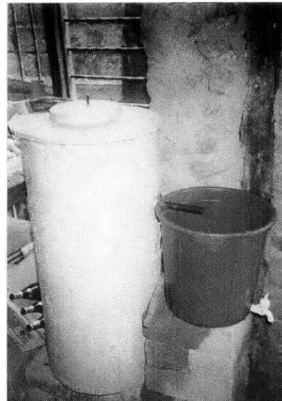
Figure 7: Concrete BSF with round base.
