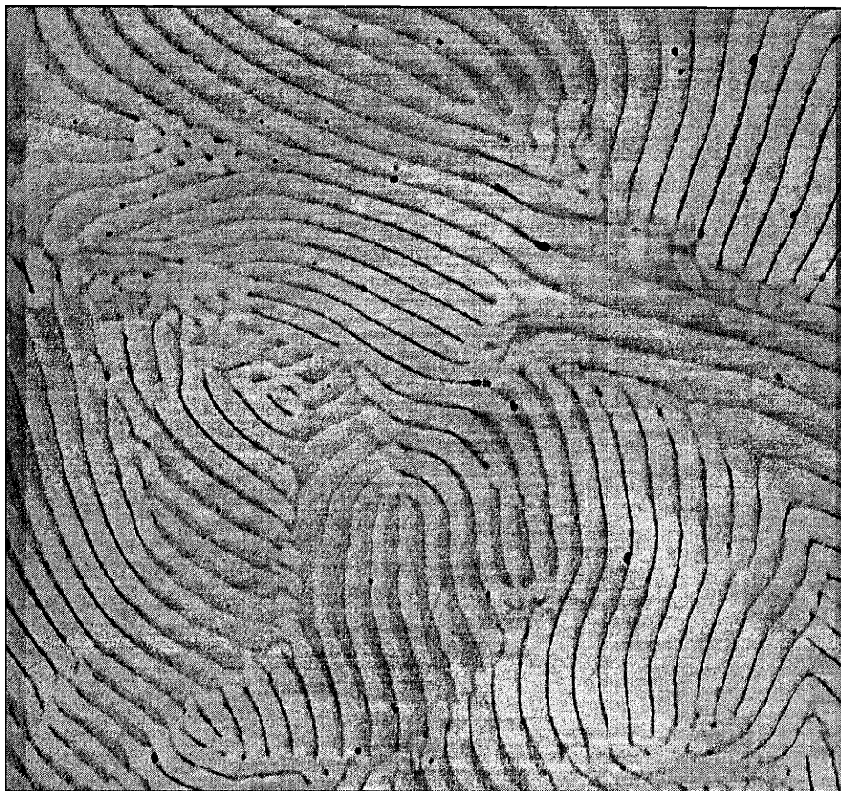
Figure 2.1A: Bulk morphology of poly(MTD 400 -NORCOOH 50 ) film cast from THF; film loaded with Na 2 (PdCl 4 ) aq
