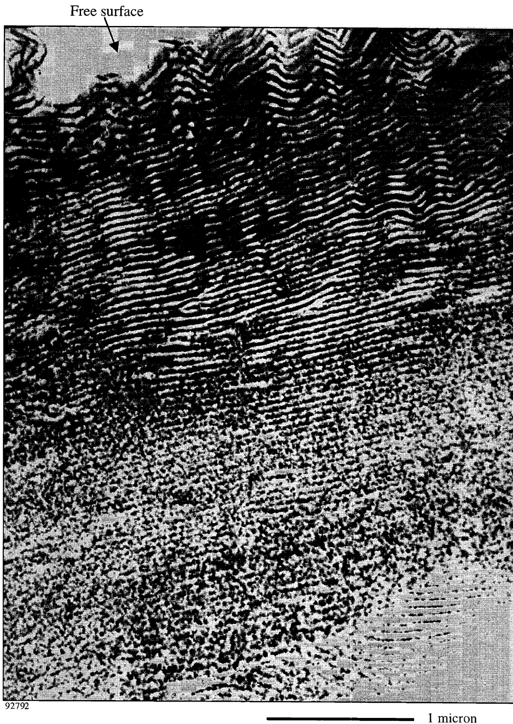
Figure 2.4: Selective electroless copper deposition via treatment in 'slow-plating' Formula II electroless copper bath for 16 hours
