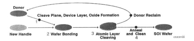
This process requires 40% fewer steps than competing wafer bonding processes and that no additional polishing, edge smoothing or damage removal steps are required, reducing complexity and producing cost savings between 50 and 70%. Note the smoothness of the as-cleaved surface on the left side of the picture below:
