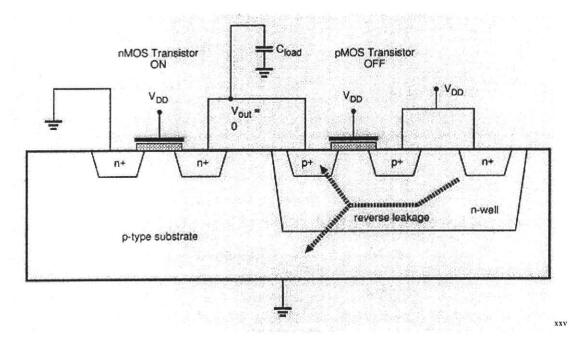
When the transistors are switched on and off in the opposite way, there is another leakage current in the nMOS transistor. When both transistors are off, there is double the leakage current. The generalized expression for the reverse current leakage in a pn junction is:
