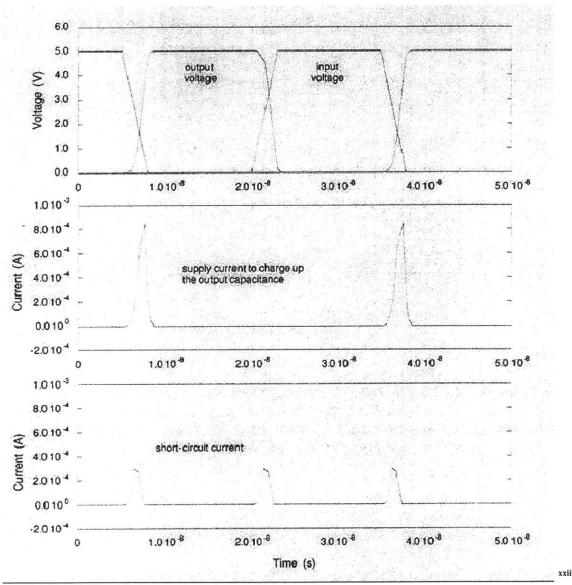
Therefore, we wish to minimize the time it takes to reach the desired input and output voltages or to sufficiently space the signals. Nevertheless, the problem still exists that there is a current draw (and therefore a power draw). The generalized expression for power consumption due to the short circuit effect is<sup>9</sup>:
