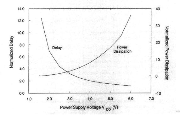
However, the propagation delay limits the switching frequency, so that the frequency is sometimes lower than expected.
